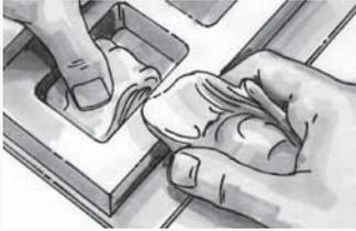
Castaldo Silicone Molding Rubber is soft and pliable, with a consistency like putty or molding clay.
