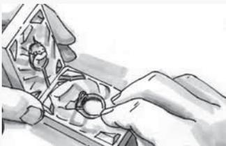
Parting lines are easily controlled and corrected by hand when used with the powder separation technique.
