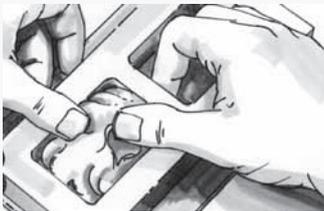
Curing Castaldo Silicone Jewelry Molding Rubber Molds involves no mixing, limited working times or de-bubbling. Simply put it in your vulcanizer at 330°-150°F (165°-177°C) for 15 minutes per 1/4 inch (6mm).
